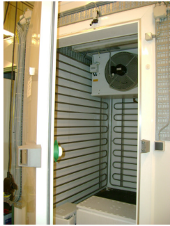
Figure 5. Styrofoam box in a cooling chamber used for cooling experiments with the agar cylinder.
